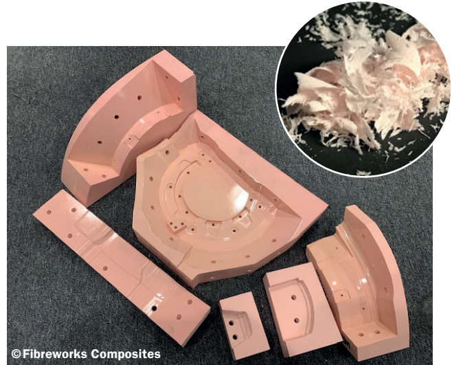
TC760X - Inset shows Flakes Produced by Profiling Bit
